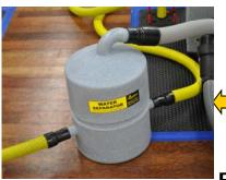
**STEP 2:** Connect up to two of the drying lines to the Water Separators two ports (cap off unused port with end cap plug). We recommend using this method for the first 24 hours after thoroughly extracting with a truck mount (see Water Separator manual).
