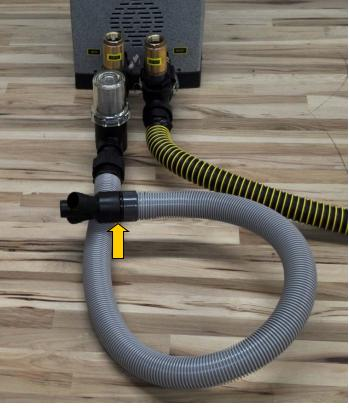
**STEP 2:** Remove and set aside the Main W from the end of the Main Air IN hose from either the HP unit.
