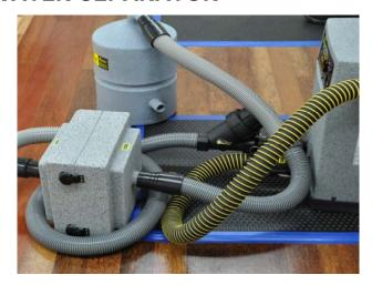
**STEP 1:** If using the Water Separator, before you connect the Interceptor Main Air IN hose to the Interceptor, thread the 2" female fitting (on the end of the Interceptor AIR IN hose) onto the 2" male fitting installed on Water Separator. Push the hose cuff onto the Interceptor.
