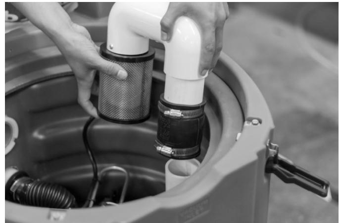
If you are servicing the float ball assembly, use a Philips screwdriver to remove the float ball housing retaining screw and remove the float ball housing. Rinse all components clean and ensure float ball moves freely inside housing. Reinstall float ball housing.
