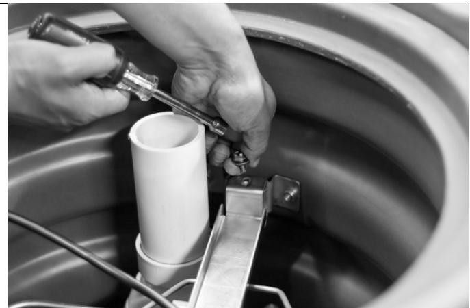
Inspect float assembly. Check float and float shaft and float switch arm for smooth operation. Clean as necessary.
