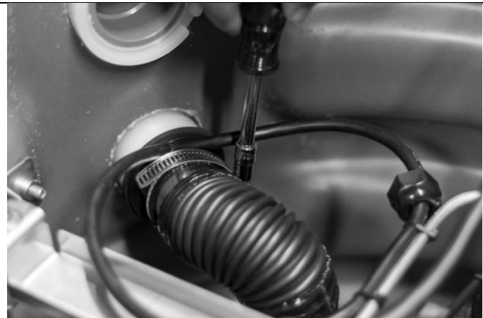
Using the 3/8 in. socket, Remove bolts on both ends of the cross-brace. Lift off brace.
