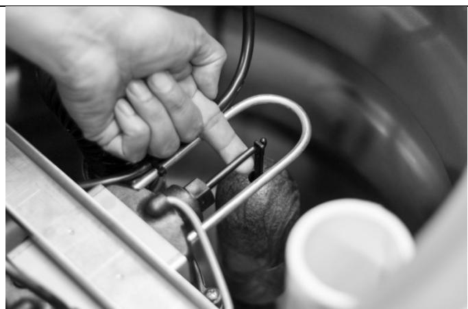
Fold up the pump handle and lift out the pump for inspection. Rest the pump on a table or other stable surface placed next to the unit. There is no need to disconnect the wire harness.
