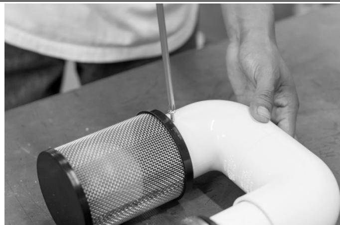
Loosen upper pump outlet hose clamp and pull the hose off the outlet.
