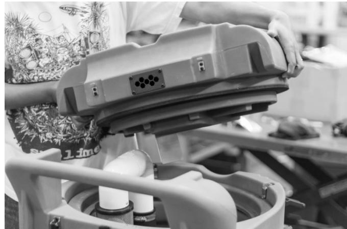
Loosen cord clamp on inside wall of tank with the 15/16 in. wrench, and pull in approximately two feet of cord or until the cord shows resistance.
