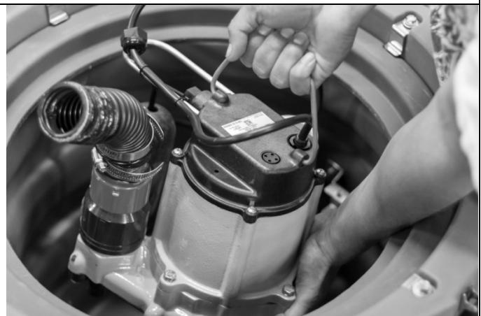
Using a Philips screwdriver, remove the pump intake cover retention screw and the plate from the bottom of the pump. Clean off any debris from intake area. Replace plate when finished.
